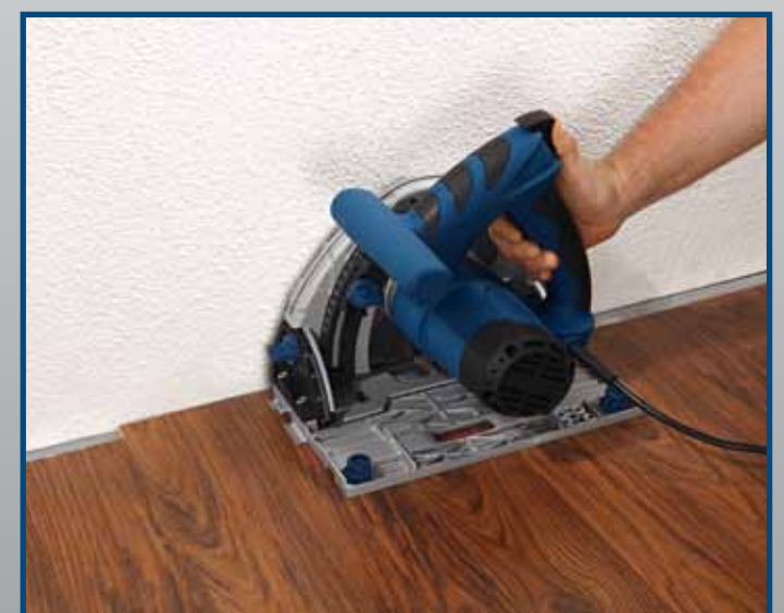
Ideal for edging up to 15.5 mm from the wall. Another example of cs 55 diverse operations.
