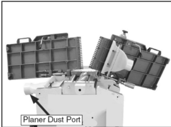
Figure 24. Planer dust port in "down" position.
