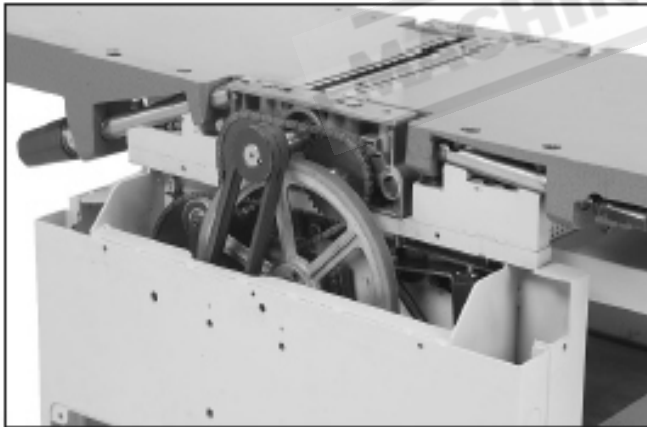
Figure 46. Fence and V-belt cover removed.
