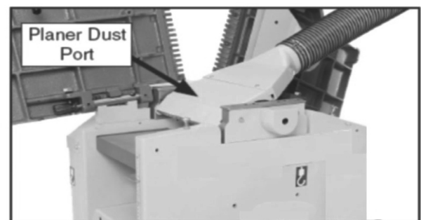
Figure 23. Planer dust port setup.
