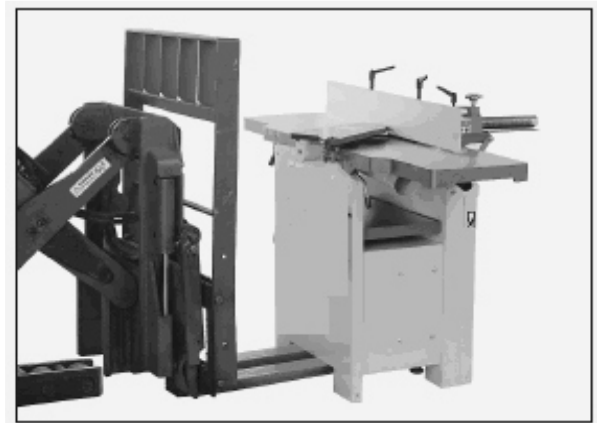
Figure 5. Lifting model with a forklift.
