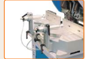
3-way material clamp switch - On & Off or Auto mode
