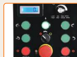
Control Panel with Digital Speed Readout
