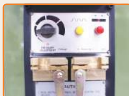
Blade Welder Unit
