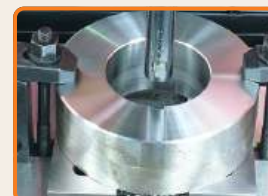
Shown Slotting Keyway with Optional Clamps & Tooling
