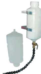
CB-2 - GRAVITY FEED COOLANT SYSTEM • Retrofit to most drilling & milling machines • Includes 2 x 1 litre plastic bottles, flex hose nozzle, flow control valve & 2 x support brackets
